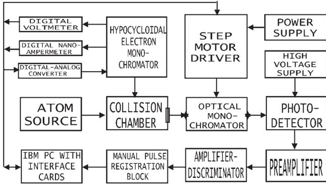
Fig. 1. The experimental apparatus layout
