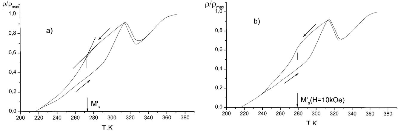
Fig. 2. Temperature dependences of the electroresistance  $R$  of a specimen made of the Ni—Mn—Ga alloy annealed at 973 K for 12 h, at (a)  $H = 0$ ; the intersections of the straight lines shown in the figure correspond to the temperatures  $M'_s$  and  $A'_s$ ; and (b)  $H = 10$  kOe
