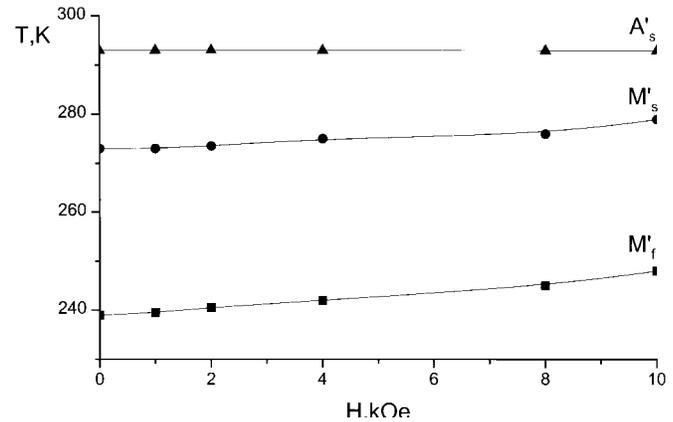
Fig. 3. Dependences of the characteristic temperatures of the intermartensitic transformation in an annealed specimen on the field value.  $M'_f$  is the final temperature (at cooling) of the intermartensitic transformation
