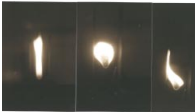
Fig. 3. General view of flame in an electric field, left to right: without field, with a field of 0.5 kV/cm, with a field of 1.5 kV/cm
