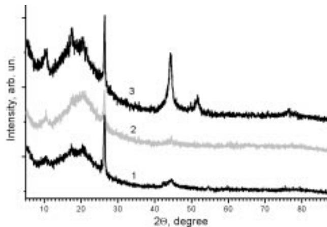
Fig. 3. X-ray powder diffraction data for soots obtained without injection of any substance (1), with the injection of Fe (2) and Ni (3)
