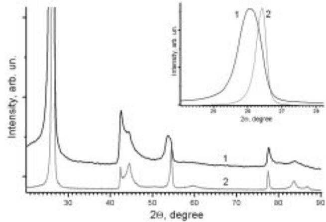
Fig. 1. X-ray powder diffraction data of thermolysis residual obtained at the feeding by current with a frequency of 50 Hz (1) and initial graphite (2)
