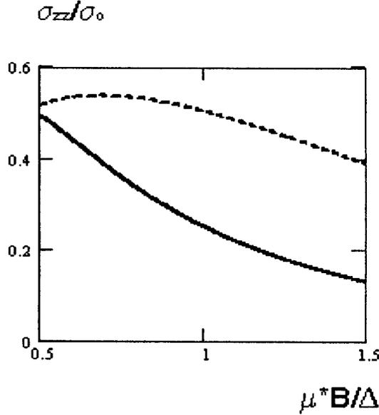
Fig. 4. Field dependence of the total conductivity at  $\gamma = 1$  calculated with taking account of the FS contraction along the magnetic field direction
