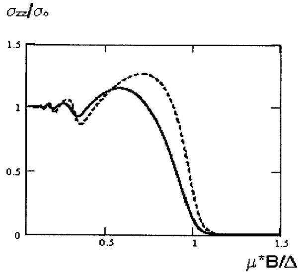
Fig. 3. Field dependence of the total conductivity in strong (ultraquantum) fields at  $\gamma = 1$  calculated without taking account of the field dependence of the chemical potential (the dashed line corresponds to the case where relaxation time is constant)
