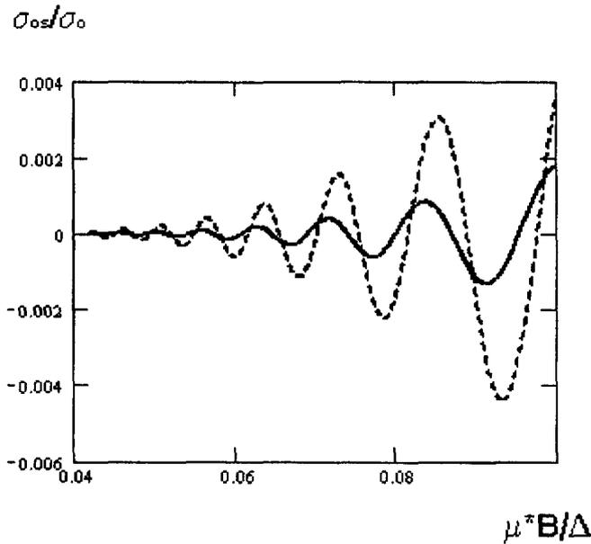
Fig. 2. Field dependence of the oscillating term of LC in weak (quasiclassical) magnetic fields (the dashed line describes the case where the relaxation time is constant)
