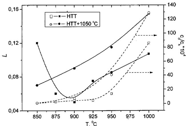
Fig. 4. Static Debye–Waller factor  $L$  (continuous curves) and relation  $c_D/c_K$  (dashed ones) vs the heat treatment temperature
