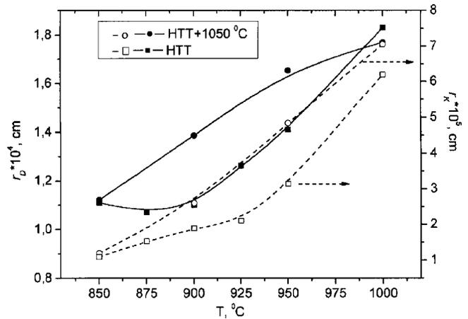
Fig. 3. Radii of dislocation loops  $r_D$  (continuous curves) and clusters  $r_K$  (dashed ones) vs the heat treatment temperature
