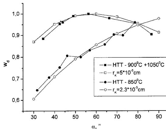
Fig. 6. The experimental and theoretical (constructed by fitting) dependences of the diffusion peak half-width on the turn angle of an analyzer
