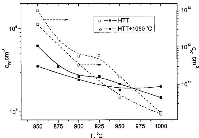
Fig. 5. Concentrations of dislocation loops (continuous lines) and clusters (dashed ones) vs the heat treatment temperature
