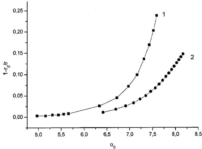
Fig. 2. Dependences of the relative errors of the calculation of the radii for clusters (1) and dislocation loops (2)
