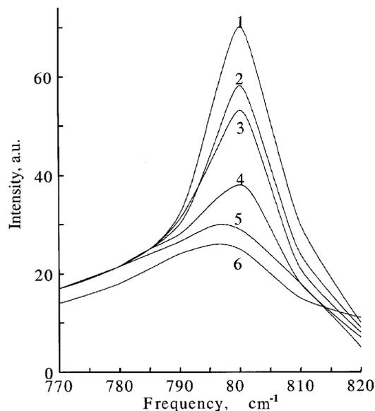
Fig. 2. Influence of the neutron irradiation dose  $F$  on the IR spectra of quartz in the frequency range  $750\text{--}850 \text{ cm}^{-1}$ :  $F = 0$  (1),  $2 \times 10^{19} \text{ cm}^{-2}$  (2),  $3 \times 10^{19}$  (3),  $4 \times 10^{19}$  (4),  $5 \times 10^{19}$  (5), and  $7 \times 10^{19}$  (6)
