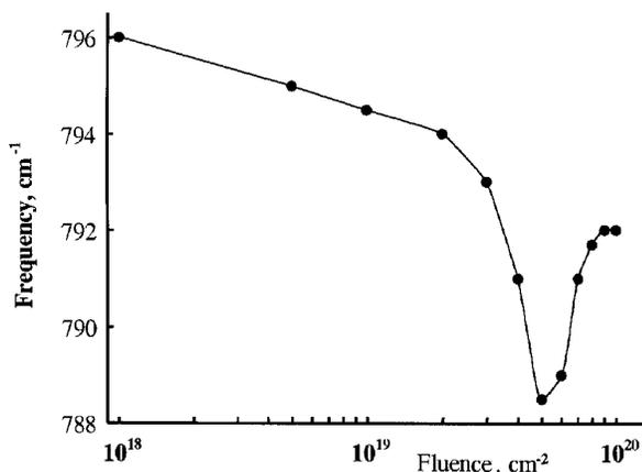
Fig. 3. Dose dependence of the maximum position of the absorption line for symmetric valence vibrations of the crystal
