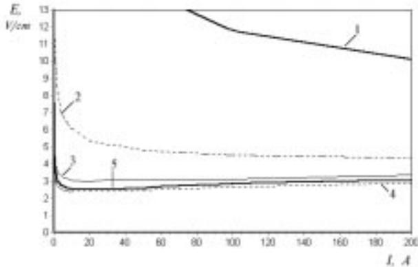
Fig. 1. Volt-ampere ( $E - I$ ) characteristics of arc discharges ( $p=1$  atm.,  $R=0.75$  cm). Curve 1 is the result of calculations for He, 2 - Ne, 3 - Ar, 4 - Kr, 5 - Xe
