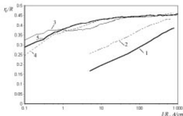
Fig. 5. Reduced radius of contraction  $r_0/R$  of an arc discharge vs the reduced current  $I/R$  ( $p = 1$  atm.). 1 - He, 2 - Ne, 3 - Ar, 4 - Kr, 5 - Xe
