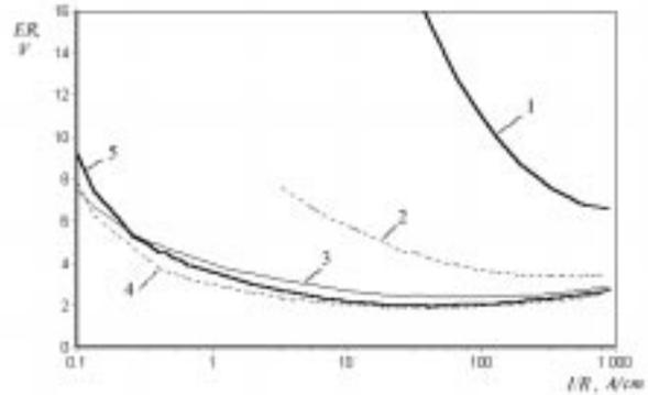
Fig. 2. Unified volt-ampere  $ER - I/R$  characteristics of arc discharges ( $p=1$  atm.). Curve 1 is the result of calculations for He, 2 - Ne, 3 - Ar, 4 - Kr, 5 - Xe
