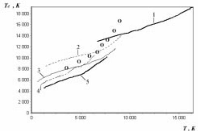
Fig. 3. Electron and gaseous temperatures in the arc ( $p=1$  atm.,  $R=0.75$  cm). 1 - He, 2 - Ne, 3 - Ar, 4 - Kr, 5 - Xe. Points  $\circ$  correspond to the experimental data for Ar [21]
