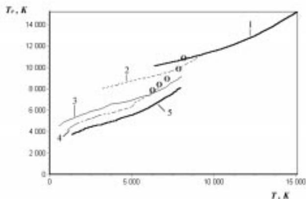
Fig. 4. Electron and gaseous temperatures in the arc ( $p = 1$  atm.,  $R = 7.5$  cm). 1 - He, 2 - Ne, 3 - Ar, 4 - Kr, 5 - Xe. The points O correspond to the experimental data for Ar [21]
