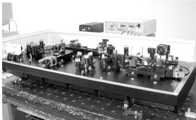
Fig. 15. A pilot device HOLO-1 (Ekspla Co.) for nondestructive control of bulk crystals, based on DFWM at 1.06 \mu\text{m}
