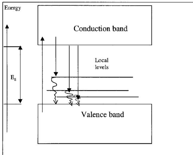
Proposed mechanism for millisecond impulse hologram recording — photoinduced recharging of local levels in the band gap
