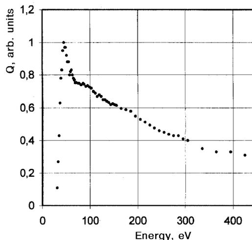
Fig. 2. Excitation function of the  $\lambda 91.98$  nm line which corresponds to the transition from the level  $3s 3p^6 {}^2S_{1/2}$
