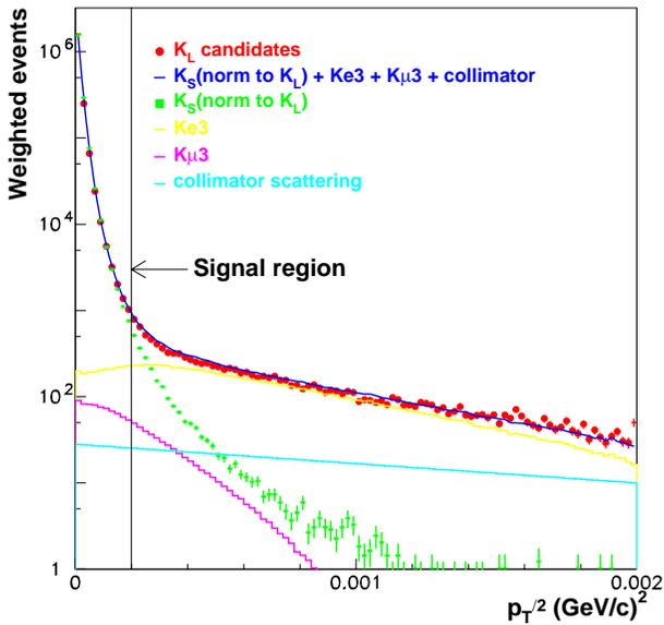
Fig.5. Distribution of  $p_T'^2$  in the charged decay mode: for weighted  $K_L$  candidates (red), background free  $K_S$  normalized to  $K_L$  and for the backgrounds arising from  $K_{e3}$  and  $K_{\mu 3}$  decays and from the scattering of a beam in the collimators
