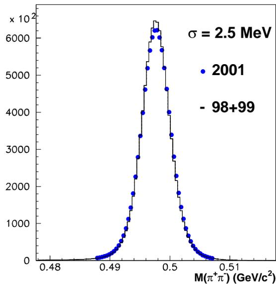
Fig.4. Distribution of the invariant masses of hadrons of positive and negative charges from selected events. The distributions obtained from 1998+1999 and from 2001 data are shown separately
