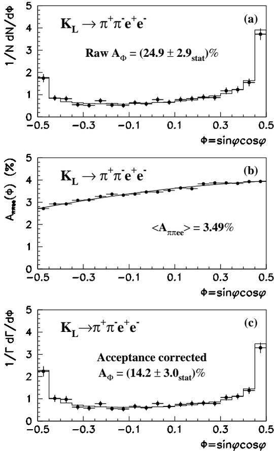
Fig. 13. *a* – distribution of the variable  $\sin\phi\cos\phi$  for  $K_L \rightarrow \pi^+\pi^-e^+e^-$  events. *b* – acceptance as a function of  $\sin\phi\cos\phi$ . The line is a polynomial fit. *c* – distribution of the variable  $\sin\phi\cos\phi$  for  $K_L \rightarrow \pi^+\pi^-e^+e^-$  events after acceptance correction. In *a* and *c* histograms are Monte Carlo predictions
