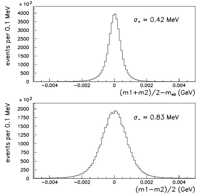
Fig.2. Distribution of the deviation of the average invariant mass of photon pairs from the  $m_{\pi^0}$  (upper plot) and of the difference of the invariant masses of photon pairs (lower plot)
