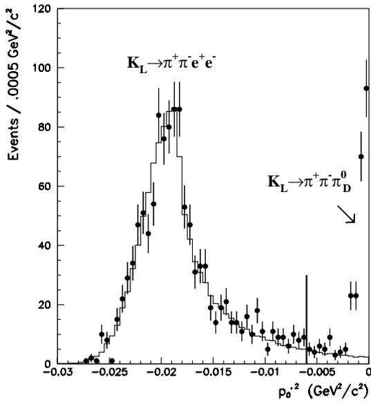
Fig. 10. Distribution of the  $p_0'^2$  variable for the selected  $K_L \rightarrow \pi^+\pi^-e^+e^-$  candidates (points). The histogram shows the distribution obtained from the  $K_L \rightarrow \pi^+\pi^-e^+e^-$  Monte Carlo events normalized to the number of observed candidates. The enhancement at  $p_0'^2 \sim 0$  is due to  $K_L \rightarrow \pi^+\pi^-\pi_D^0$  decays. The signal region is defined to the left from the vertical line
