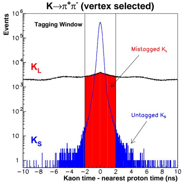
Fig.6. Distribution of the difference of the decay time of  $K_S$  (blue) and  $K_L$  (red) into charged pions and the nearest proton time measured in the tagger.  $K_S$  and  $K_L$  were identified using their vertex positions
