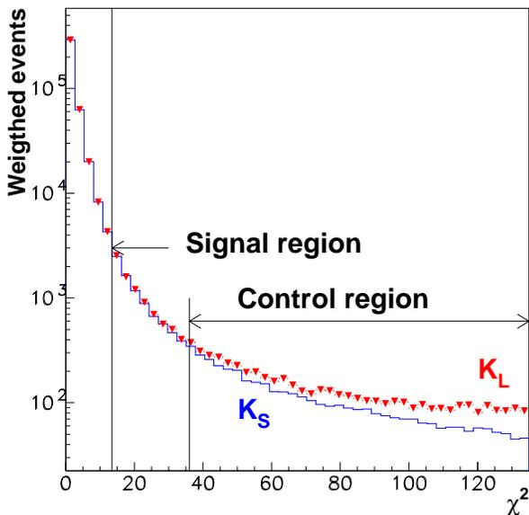
Fig.3. Distribution of  $\chi^2$  in the neutral decay mode: for the weighted  $K_L$  candidates (red points) and the background free  $K_S$  decays. Background in  $K_L$  is estimated in the control region and extrapolated to the signal region.
