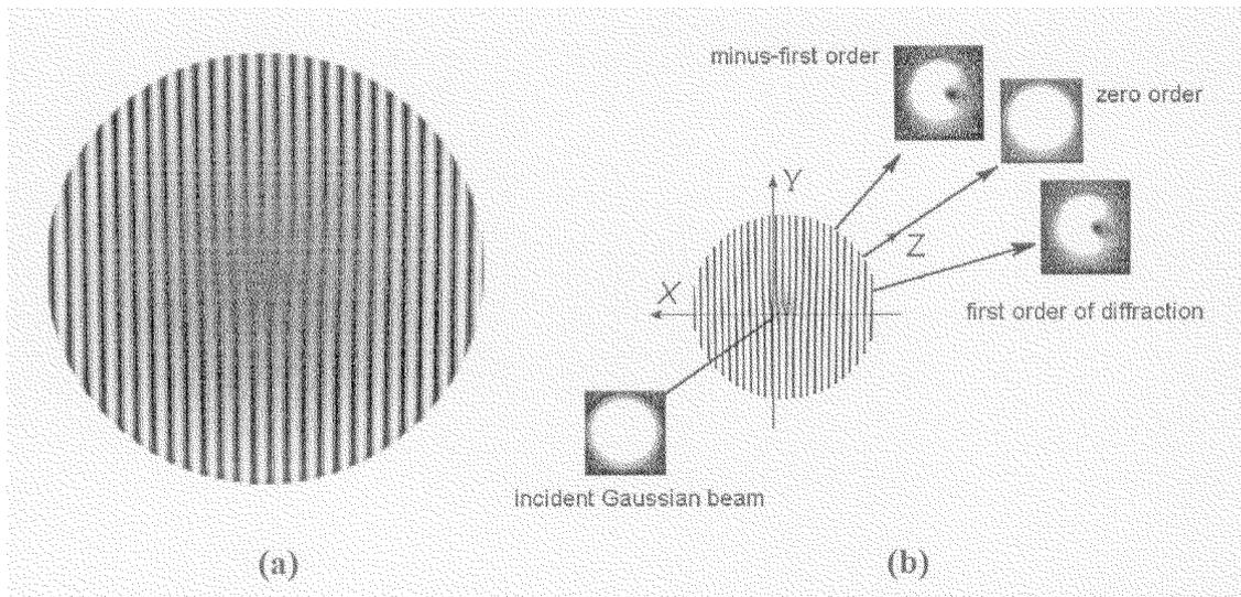
Fig. 1. *a* - example of a computer-synthesized hologram suitable for OV beam production in the first diffracted order: grating with linear modulation of the fringes contrast, developed for the  $LG_0^1$  mode creation,  $M = 1$ . *b* - schematical representation of the diffraction by the grating displaced with respect to the readout Gaussian beam. Diffracted beams in the near field are shown
