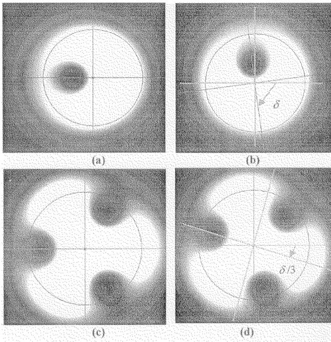
Fig. 2. Views of the beam spot in the one-beam interferometer for zero phase difference between the Gaussian and vortex components (left column) and for phase difference  $\delta$  (right column). The OV charge in the vortex component equals 1 (a, b) and 3 (c, d). The Z-axis is directed towards the reader
