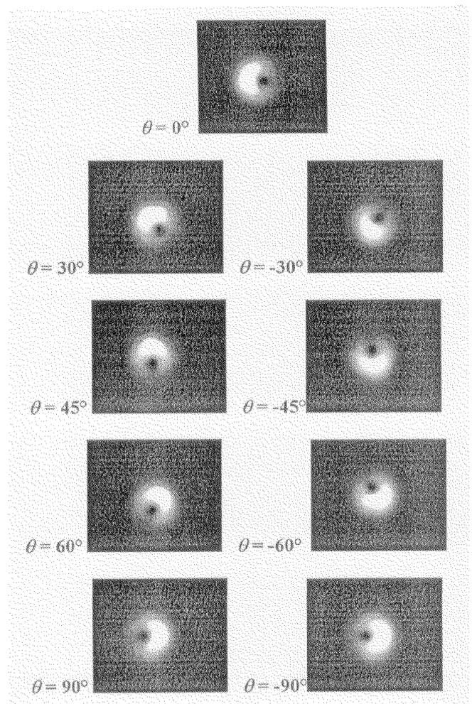
Fig. 4. Experimental observation of the off-axis OV rotation in the one-beam interferometer (scheme shown in Fig. 3)
