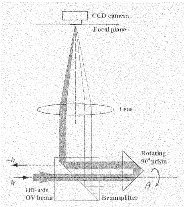
Fig. 3. Back-reflection scheme with the  $90^\circ$  prism, rotating around the axis of the incident beam. The retro-reflected beam is directed by a beam-splitter to the focusing spherical lens. Independently on the angle of the prism orientation, the beam will come to the same spot in the focal plane of the lens, where the CCD camera is placed. The beam path for the angle  $\theta = 0$  (shaded area) is shown, the beam path for the angle  $\theta = 180^\circ$  is also shown
