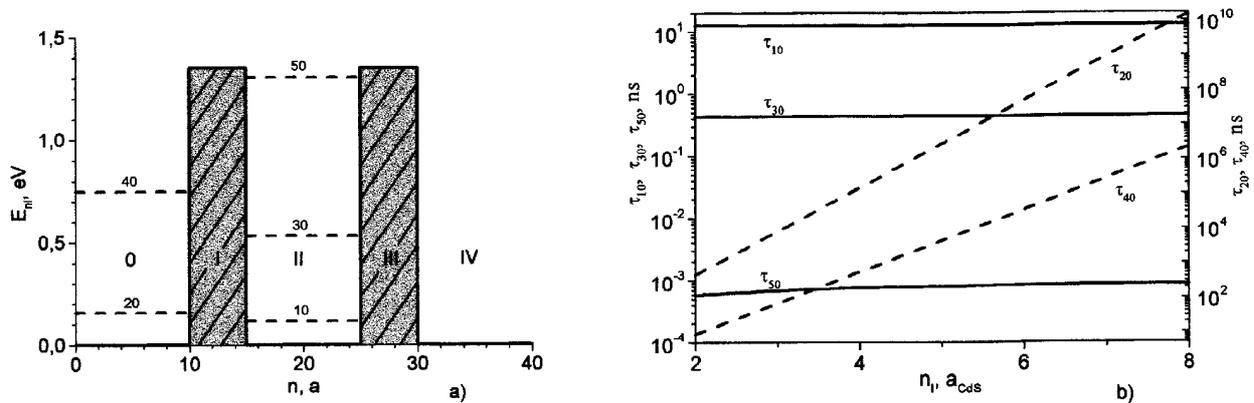
Fig. 5. Scheme of electron potential energy location of resonance levels (a) and electron lifetimes dependences on barrier thickness  $\Delta_1$  at  $n_0 = 15$ ,  $\Delta_2 = 15$ ,  $\Delta_3 = 5$  (b)
