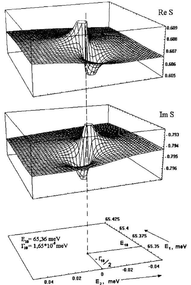
Fig. 2. Dependences of the real and imaginary parts of the scattering matrix  $S$  on  $\tilde{E}$  and location of the pole in the complex plane for state  $|100\rangle$  at  $n_0 = 15$ ,  $\Delta_1 = 5$ ,  $\Delta_2 = 15$ ,  $\Delta_3 = 5$  in units of lattice constant
