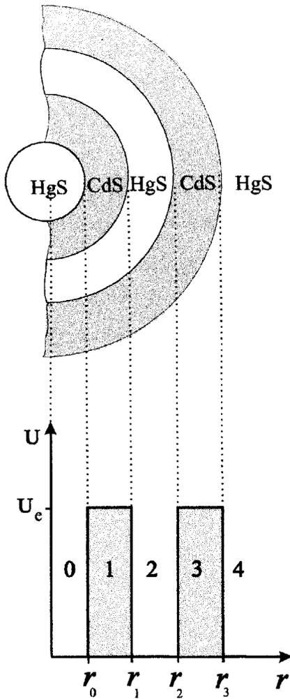
Fig. 1. Geometric scheme (a) and electron potential energy scheme (b) for the spherical nanosystem
