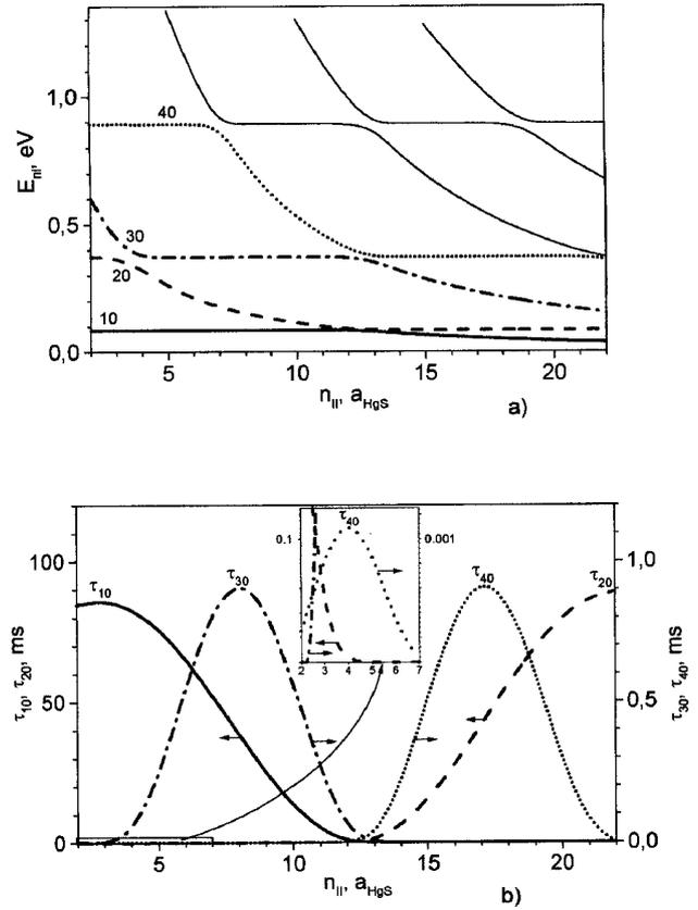
Fig. 4. Dependences of electron resonance energies  $E_{n0}$  and lifetimes  $\tau_{n0}$  on  $\Delta_2$  at  $n_0 = 15$ ,  $\Delta_1 = 5$ ,  $\Delta_3 = 5$
