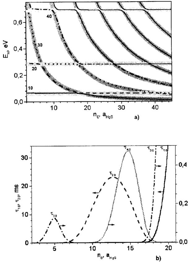
Fig. 3. Dependences of electron resonance energies  $E_{n0}$  and lifetimes  $\tau_{n0}$  on  $n_0$  at  $\Delta_1 = 5$ ,  $\Delta_2 = 15$ ,  $\Delta_3 = 5$
